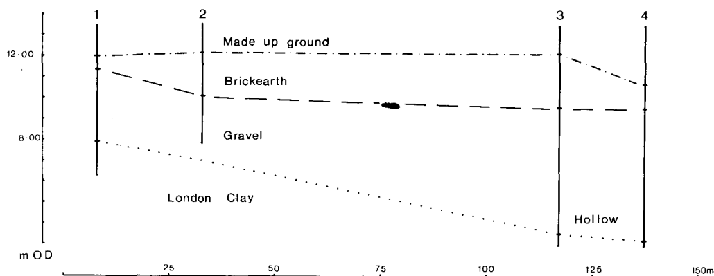
Fig. 12. Paternoster Square and Warwick Square: Boreholes and reconstructed geological section through drift-filled hollow.
