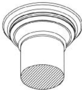
Fig 12. Reconstructed original form of pier capital of 1270–1330, stone <3336> (Fig 30, No. 13)
